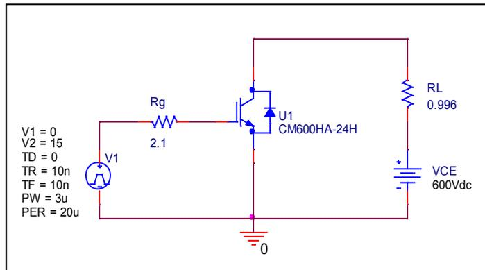
Test condition  $I_c=600$  (A),  $V_{cc}=600$ (V)
