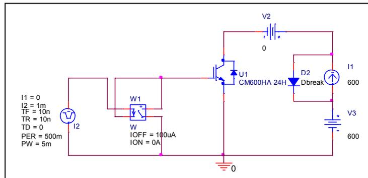
Test condition:  $V_{CC}=600$  (V),  $I_C=600$ (A) ,  $V_{GE}=15$ (V)
