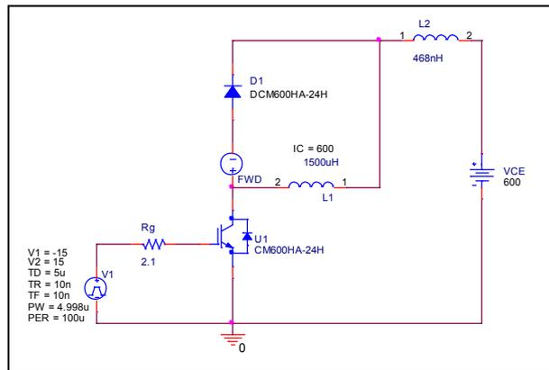
Test condition:  $V_{CC}=600$  (V),  $I_C=600$ (A) , $V_{GE}=\pm 15$ (V)
