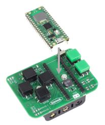
Inserting a Pico: To use the Mini Controller the Pico should have soldered pin header and be inserted firmly into the connector as shown. Note: The Pico pins will stick through the board slightly as the pin sockets are low-profile.
