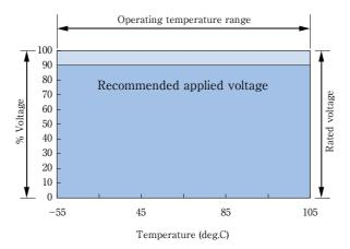
Fig.1 Explanation of recommended applied voltage
