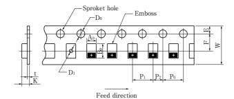
Note) Standard taping orientation is R. R indicates cathode is located to sprocket hole.
