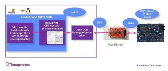
Bus Blaster can be used with various other debugging, programming and boundary scan test software, so there are a rich variety of resources available for your MIPS development project.
