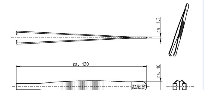
All dimensions are in mm; tolerances according to ISO 2768 m-H
