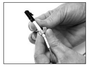
21.3 Taper on the boot will cause the yoke to spread allowing the correct placement at the rear of the connector.
