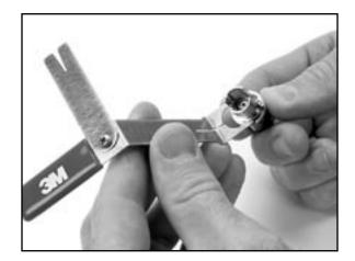
4.4 Insert the connector into the hot melt connector holder.
