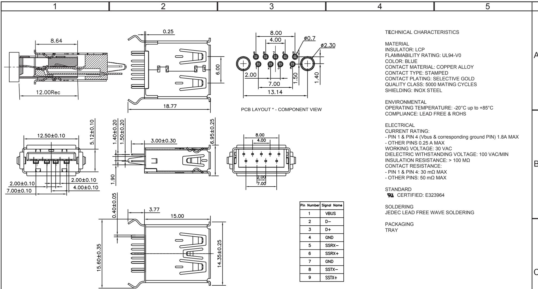
\* NOTE: THE RECOMMENDED PCB LAYOUT IS FOR AN OPTIMIZED RETENTION FORCE OF CONNECTOR ON PCB BUT IT IMPLIES INSERTION FORCE THAT A LOT OF PICK AND PLACE MACHINES ARE NOT ABLE TO HANDLE. THEREFORE IT MIGHT BE NECESSARY TO DRILL BIGGER HOLES FOR THE CLIPS. PLEASE CHECK THIS CAREFULLY.
