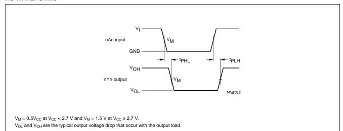
Fig.5 Input (nAn) to output (nYn) propagation delays.
