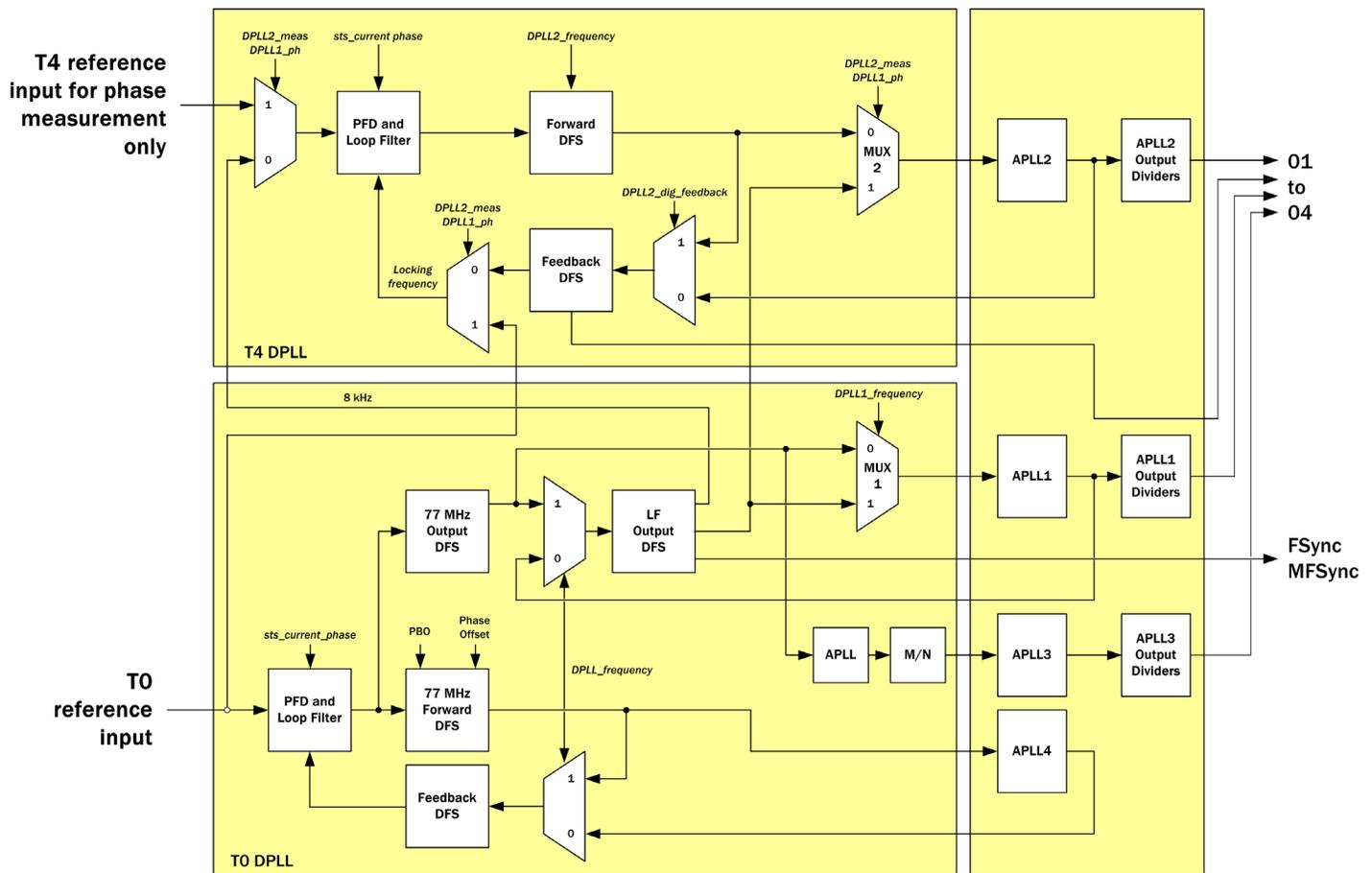
The T4 output APLL is also for multiplying and filtering. The input to the block can come from the T4 forward DFS block or from the T0 path. The input to the T4 output APLL can be programmed to be one of the following:
