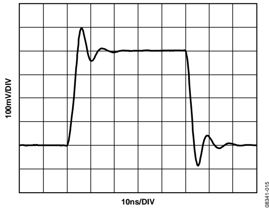
Figure 40. Small Signal Transient Response, G = 12.04 \text{ dB}
