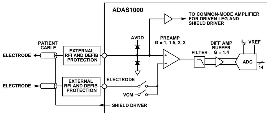
Figure 56. Simplified Schematic of a Single ECG Channel
