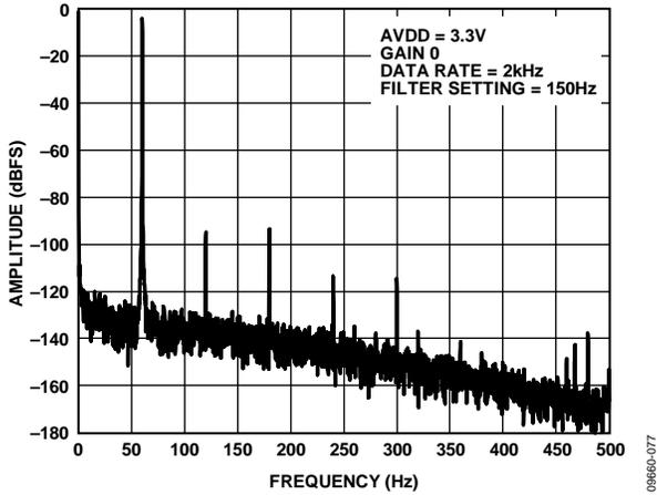
Figure 48. FFT with 60 Hz Input Signal
