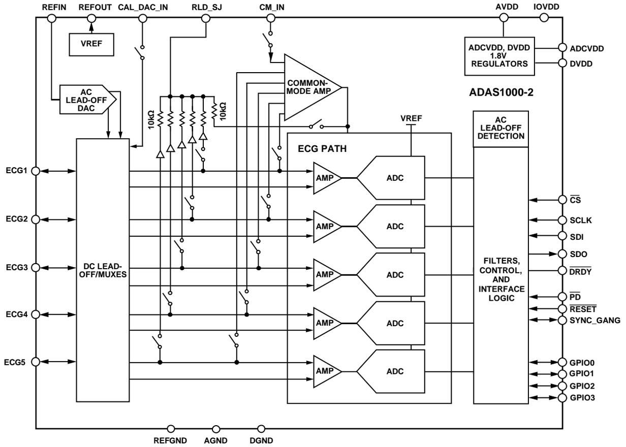
Figure 55. ADAS1000-2 Slave Device Simplified Block Diagram
