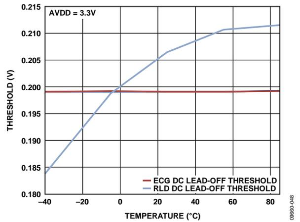
Figure 21. DC Lead-Off Comparator Low Threshold vs. Temperature
