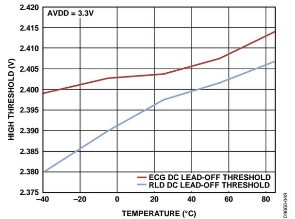
Figure 22. DC Lead-Off Comparator High Threshold vs. Temperature
