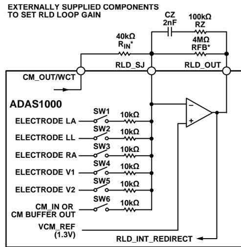
\*EXTERNAL RESISTOR R<sub>IN</sub> IS OPTIONAL. IF DRIVING RLD FROM THE ELECTRODE PATHS, THEN THE SERIES RESISTANCE WILL CONTRIBUTE TO THE R<sub>IN</sub> IMPEDANCE. WHERE SW1 TO SW5 ARE CLOSED, R<sub>IN</sub> = 2kΩ. RFB SHOULD BE CHOSEN ACCORDINGLY FOR DESIRED RLD LOOP GAIN.
