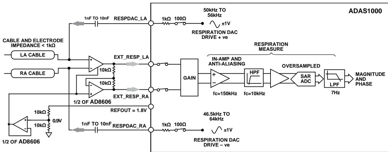
Figure 71. Respiration Using External Capacitor and External Amplifiers
