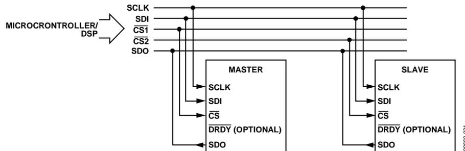
Figure 78. One Method of Interfacing to Multiple Devices
