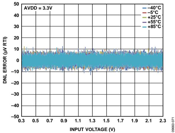
Figure 43. DNL vs. Input Voltage Range Across Temperature
