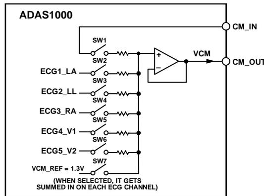
Figure 66. Common-Mode Generation Block
