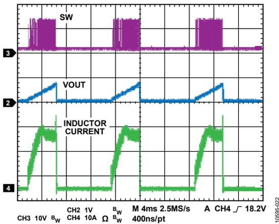
Figure 22. Current-Limit Hiccup Mode, 30 A Current Limit
