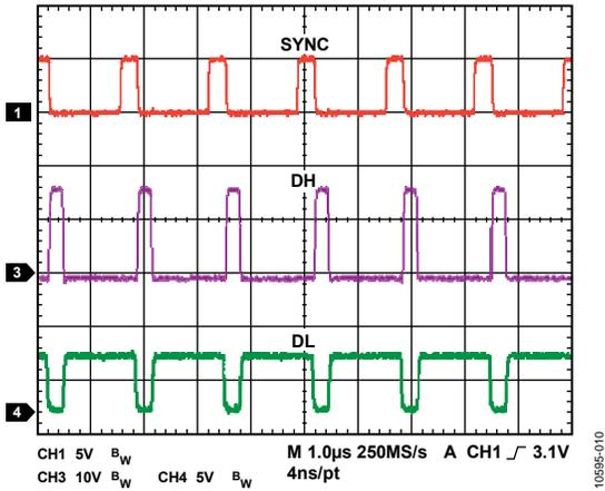
Figure 10. Synchronization,  $f_{SYNC} = 600 \text{ kHz}$
