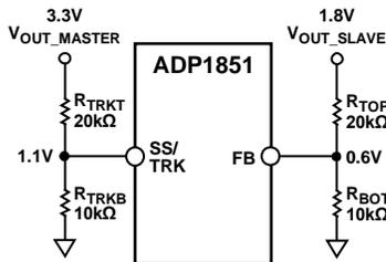
Figure 31. Example of a Coincident Tracking Circuit
