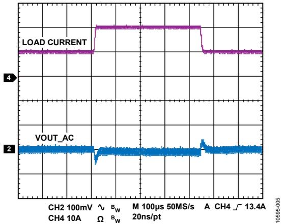
Figure 5. 10 A to 20 A Load Step,
