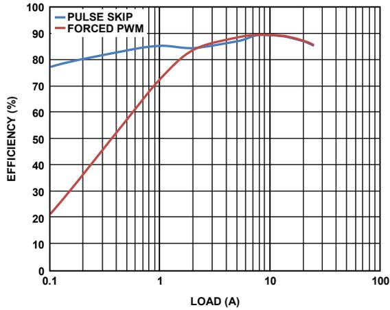
Figure 4. Efficiency Plot
