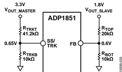
Figure 33. Example of a Ratiometric Tracking Circuit
