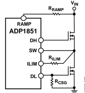
Figure 27. Slope Compensation and CS Gain Connection
