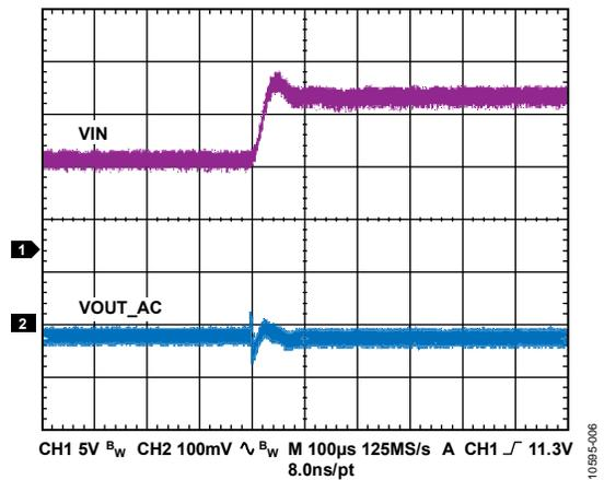
Figure 6. 9 V to 15 V Line Step,
