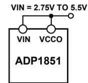
Figure 20. Configuration for  $V_{IN} < 5.5$  V
