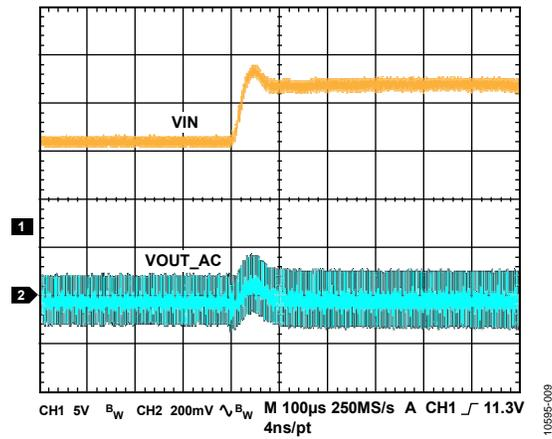
Figure 9. 9 V to 15 V Line Step,
