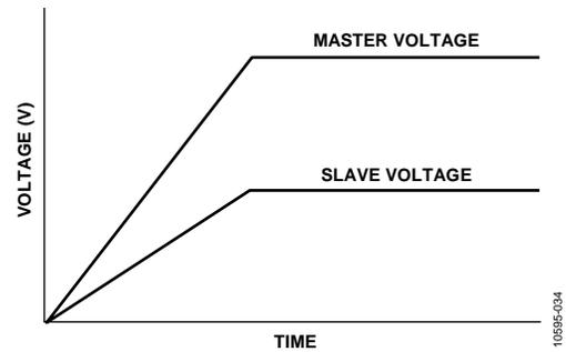
Figure 32. Ratiometric Tracking
