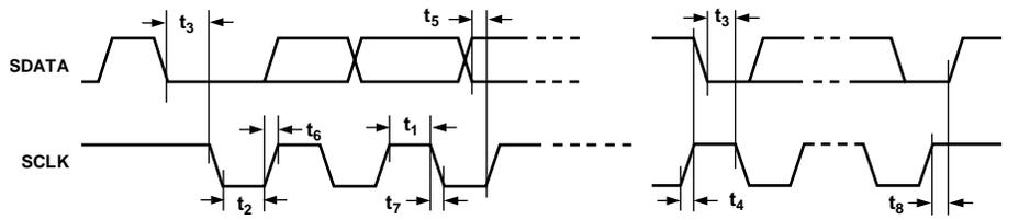
Figure 2. I<sup>2</sup>C Timing Diagram
