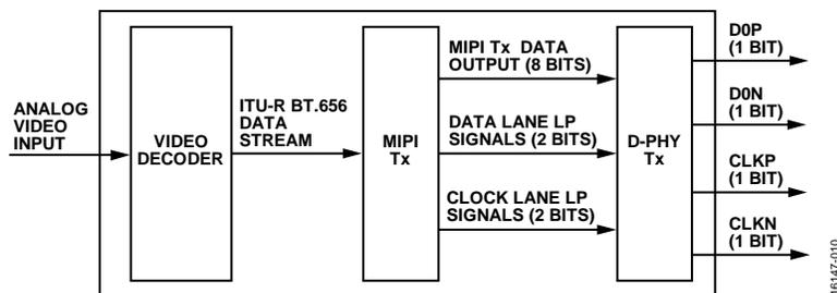
Figure 9. MIPI Tx Output Stage of the ADV7281A
