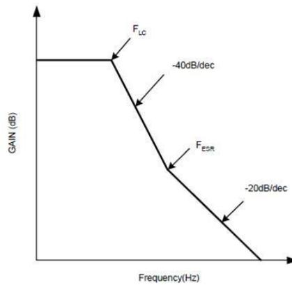
Figure 12. Frequency Response of the LC Filters
