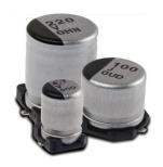
Type AVES Capacitors are rated for 1000 hours at 105 °C with low impedance characteristics. They are ideal for high density PC board packaging. The Type AVES offers a low in-place-cost for a high quality performer. The vertical cylindrical cases facilitate automatic mounting and reflow soldering into the same footprint of like-rated tantalum capacitors except without the need for voltage derating. Type AVES is RoHS compliant.
