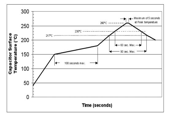
Parts should be subjected to just one reflow soldering process.
