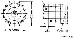
\*) This recess must be on the side of the grounding pin to ensure that the yoke locks in position.
