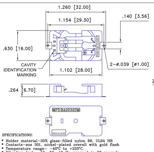
\* Vibration test 10 50 10 Hz sweeped in 60 seconds X,Y,Z direction 1 hour each direction Result: No dislodgement of the cell or damage No discontinuity over 10 micro-seconds.
