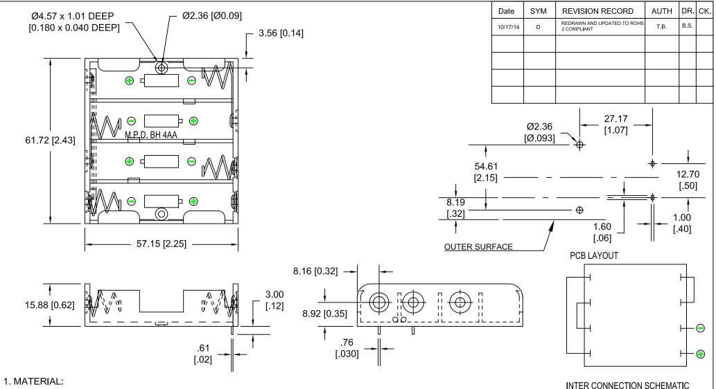
HOUSING: IMPACT NYLON 6, UL94V-0, UL FILE NO. E48285
