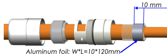
Step 4: Wrap foil over braided shielding
