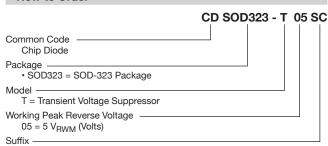
S = Standard Capacitance Unidirectional Diode SC = Standard Capacitance Bidirectional Diode
