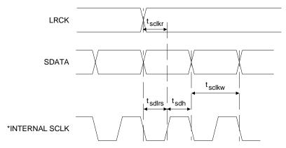
Figure 4. Internal Serial Mode Input Timing
