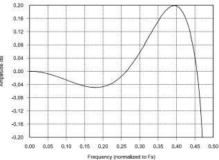
Figure 21. Double-Speed Passband Ripple
