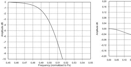
Figure 20. Double-Speed Transition Band
