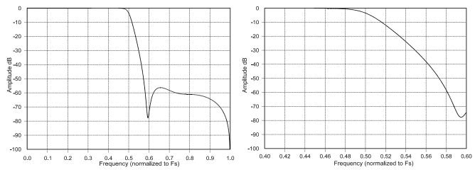
Figure 18. Double-Speed Stopband Rejection
