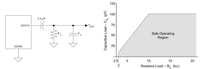
Figure 1. Equivalent Output Test Load
