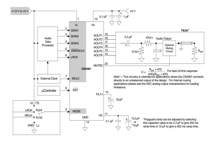
Figure 6. Recommended Connection Diagram
