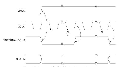
Figure 5. Internal Serial Clock Generation
