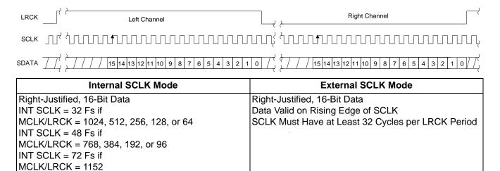
Figure 10. CS4361 Data Format (Right-Justified 16)
