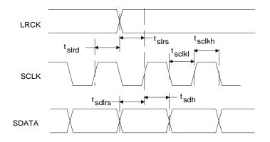
Figure 3. External Serial Mode Input Timing
