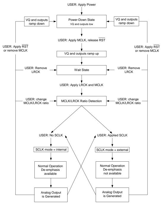
Figure 12. CS4361 Initialization and Power-Down Sequence
