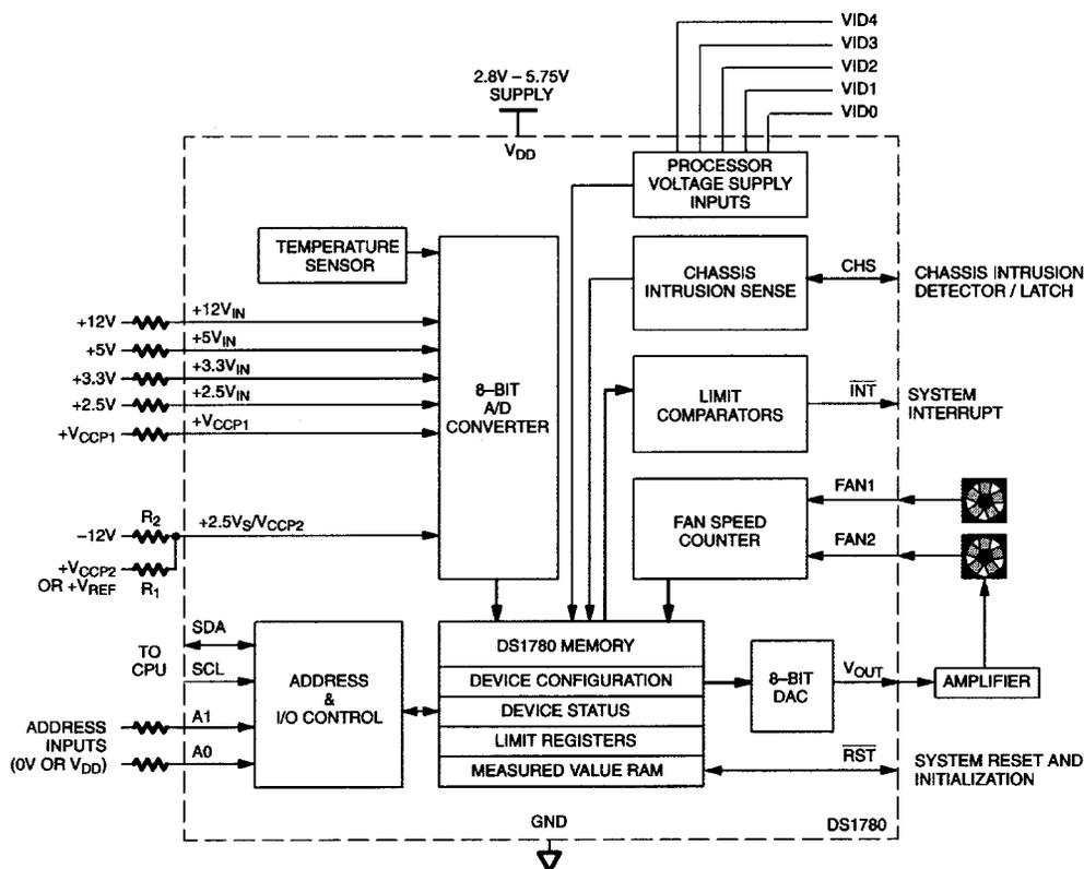
**Note:** R1 and R2 on the -12V resistance ladder should be ratioed such that approximately +2.5V appears at the input pin (i.e., R1=4k $\Omega$ , R2=23.2 k $\Omega$ ). If a second processor voltage needs to be monitored ( $V_{CCP2}$ ), leave R2 empty, and make R1 500 $\Omega$ , with  $V_{CCP2}$  appearing here.
