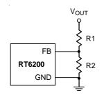
Figure 1. Output Voltage Setting
