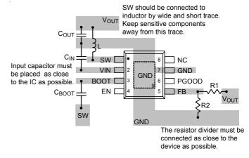
Figure 4. PCB Layout Guide
