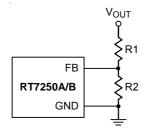
Figure 1. Output Voltage Setting
