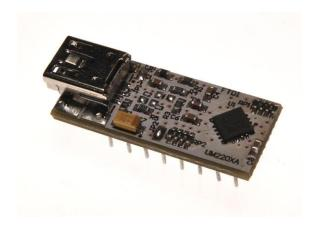
UMFT220XA is a USB to 4-bit SPI/FT1248 DIP module with a 0.3" row pitch.
