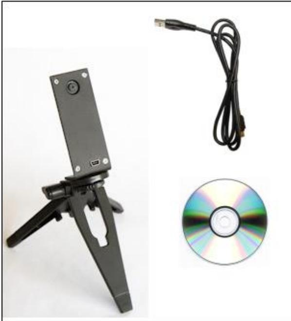
The V1KU Starter Kit includes one V1KU board with stand and a link to Image Trainer software ready to interface with the board through its USB port, as well as a Software Development Kit (SDK) for C/C++ or .Net development platforms.
