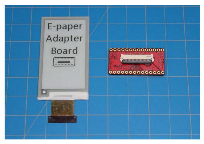
• **The E-paper Adapter**: If you are looking to integrate the E-paper board into an existing solution, you can purchase just the board by itself. Comes with just the E-paper adapter.
