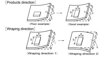
Products shall be location the sideways Direction (Length : a<b) to the machanical Stress.
