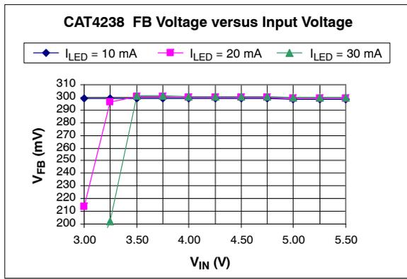
Figure 5. V<sub>FB</sub> Voltage Line Regulation
