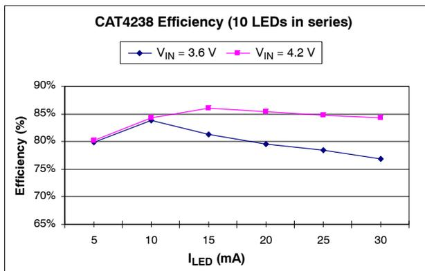
Figure 6. CAT4238 Efficiency Driving 10 LEDs in Series
