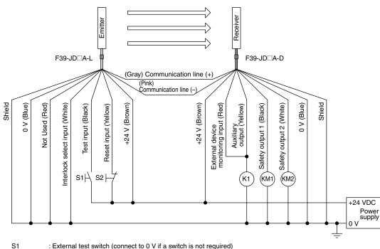
: External test switch (connect to 0 V if a switch is not required)
