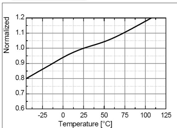
Figure 20. Output Saturation Voltage (V<sub>RDY,SAT</sub>) vs. T<sub>A</sub>
