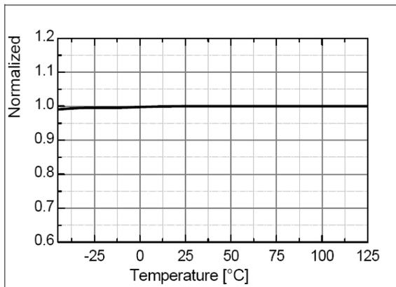
Figure 6. Stop Threshold Voltage (V<sub>STOP</sub>) vs. T<sub>A</sub>
