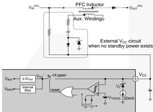
Figure 22. Startup Circuit
