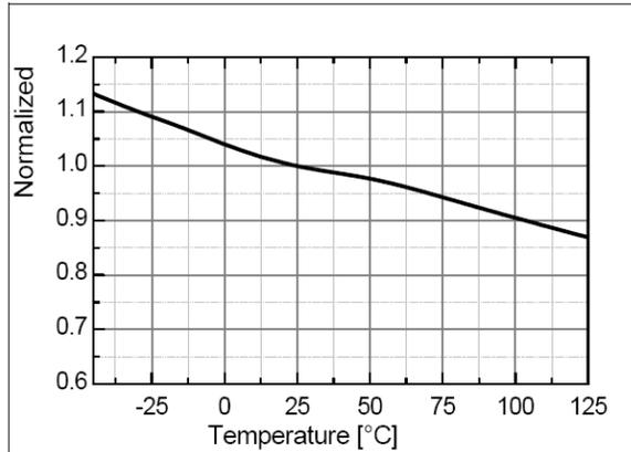
Figure 7. Startup Supply Current (I<sub>START</sub>) vs. T<sub>A</sub>
