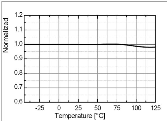
Figure 16. Output Voltage High (V<sub>OH</sub>) vs. T<sub>A</sub>
