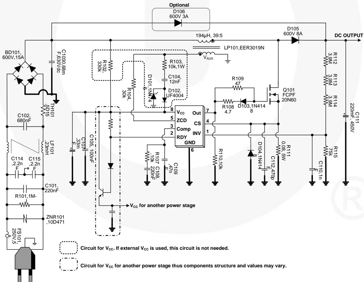
Figure 45. Demonstration Circuit
