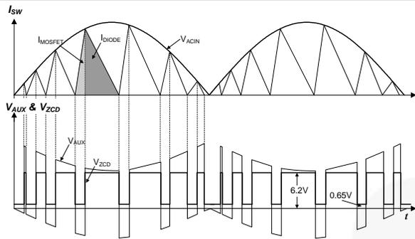
**Figure 28. Auxiliary Voltage Depends on MOSFET Switching**
