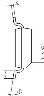
SOIC 8 Dimensions in mm
