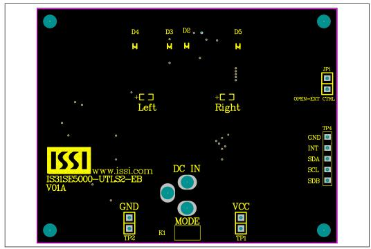
Figure 3: Board Component Placement Guide - Top Layer
