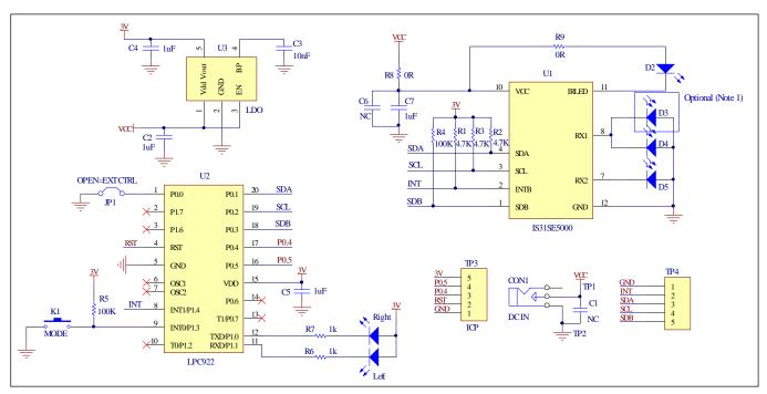
Figure 2: IS31SE5000 Application Schematic
