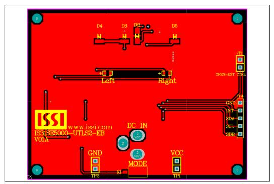
Figure 4: Board PCB Layout - Top Layer
