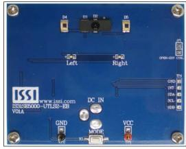
Figure 1: Photo of IS31SE5000 Evaluation Board
