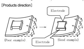
Products shall be located in the sideways direction to the mechanical stress.
