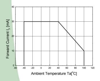
**Ambient Temperature vs. Forward Current**
