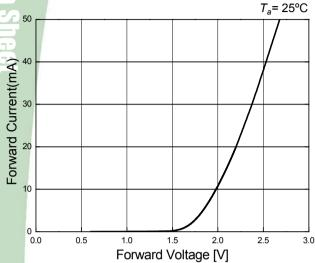
Forward Voltage vs. Forward Current
