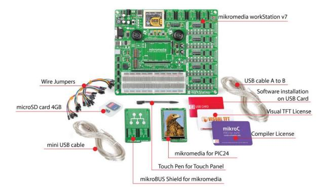
Each kit includes a mikromedia board, Visual TFT software license, compiler license, software installation on USB card, a mikroBUS Shield for mikromedia, mikromedia workStation v7, Touch pen for the screen, mini USB and USB type A to B cable, microSD card (4GB), and 30 pieces of wire jumpers.
