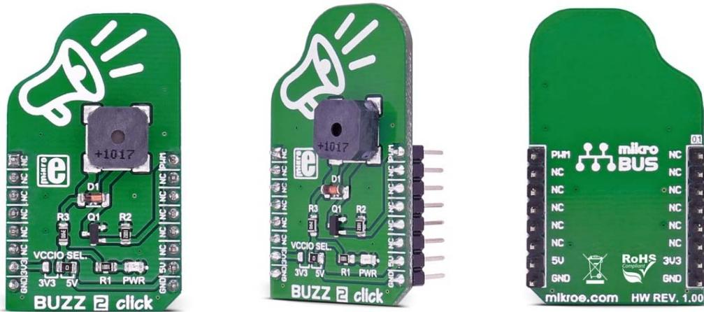
**BUZZ 2 click** carries the CMT-8540S-SMT magnetic buzzer transducer. The buzzer's resonant frequency is 4kHz. The click is designed to run on either 3.3V or 5V power supply.
