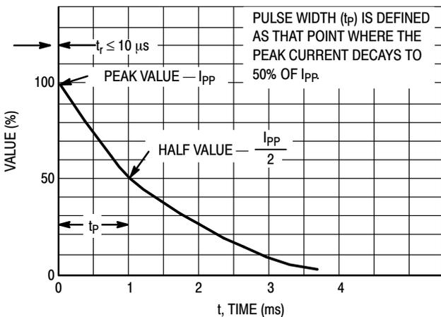
Figure 5. Pulse Waveform
