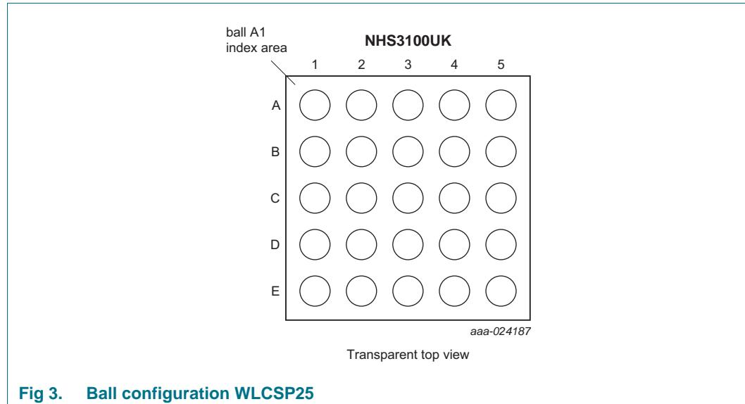
**Fig 3. Ball configuration WLCSP25**
