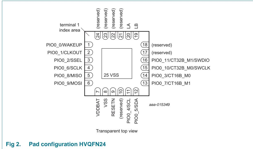
**Fig 2. Pad configuration HVQFN24**
