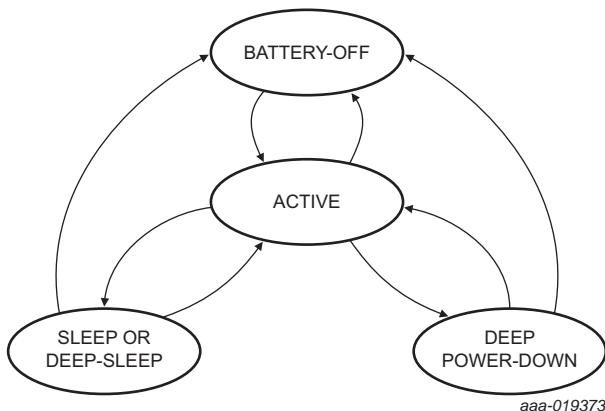
**Fig 8.** PMU state transition diagram
