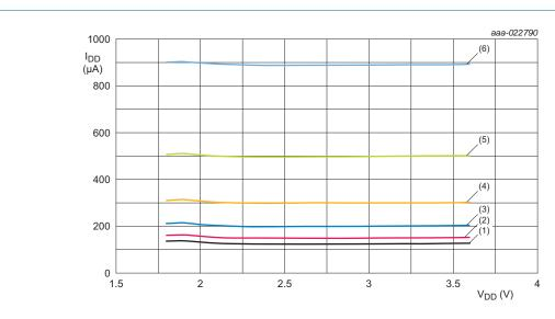
Plot of  $I_{DD} / V_{DD}$  when ARM running a while-1 loop in Normal mode, no NFC field present.
