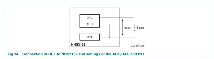
Apply the desired bias voltage to the first terminal (preferably as high as possible), and sequentially measure the voltage and current on the second terminal. The resistance is found by dividing the measured voltage drop with the measured current through the DUT.
