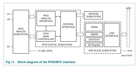
The CMDIN, DATAOUT, Status Register (SR) and SRAM are mapped in the user memory space of the RFID core. The RFID READ and WRITE commands allow wireless communication to this shared memory.
