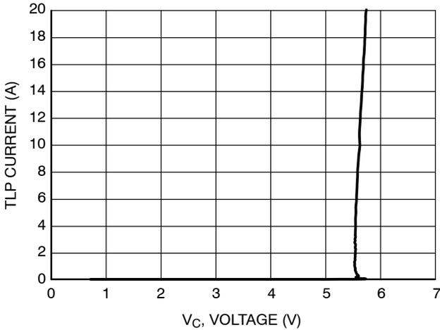
Figure 3. Positive TLP I-V Curve, Pin 2 to Pin 1
