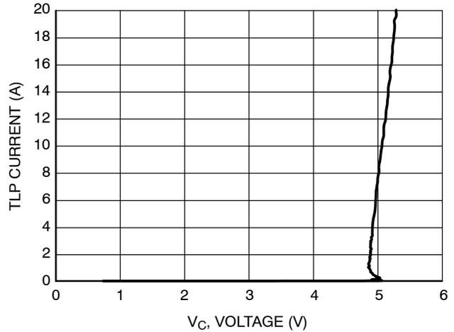
Figure 4. Negative TLP I-V Curve, Pin 1 to Pin 2
