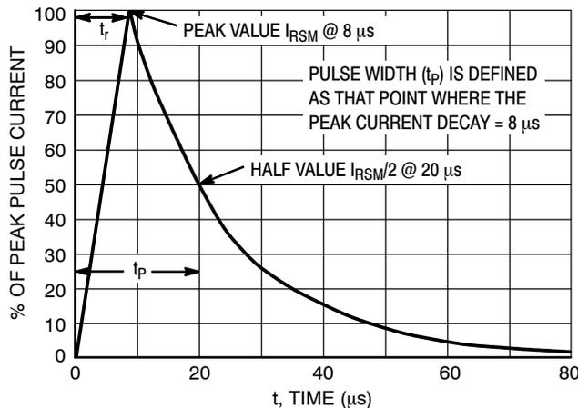
Figure 12. 8 x 20 μs Pulse Waveform
