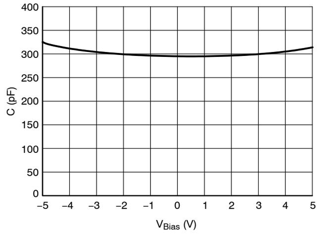
**Figure 7. CV Characteristics**
