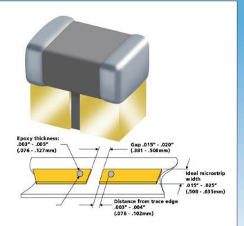
4. After the reflow step is completed, inspect joint for voids or excess flux and non-reflowed solder balls that can degrade performance or cause shorts across the gaps. Proper cleaning after the reflow process is crucial to avoiding performance degradation and discovering poor solder ioints
