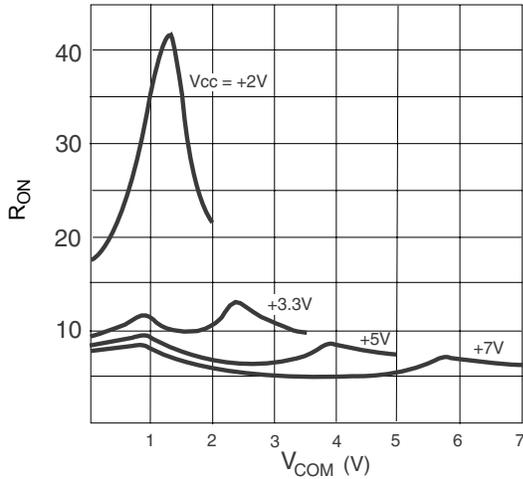
**$R_{ON}$  vs.  $V_{COM}$  and Temperature**
