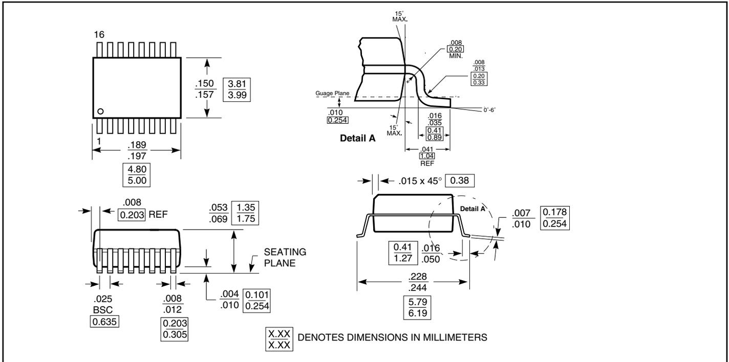
**Packaging Mechanical: 16-Pin SOIC (W)**
