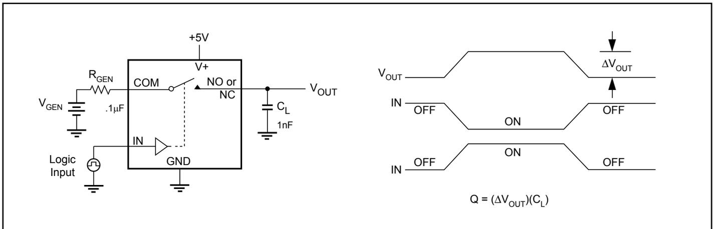
**Figure 2. Charge Injection**
