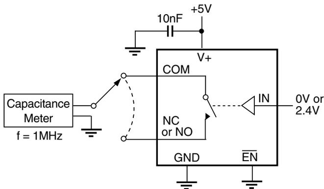
**Figure 5. Channel-Off Capacitance**
