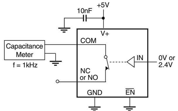
**Figure 6. Channel-On Capacitance**
