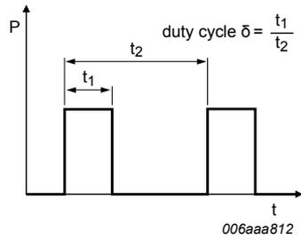
Fig. 17. Duty cycle definition
