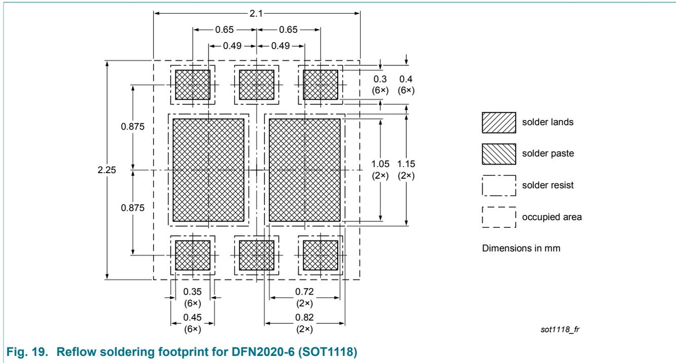
Fig. 19. Reflow soldering footprint for DFN2020-6 (SOT1118)
