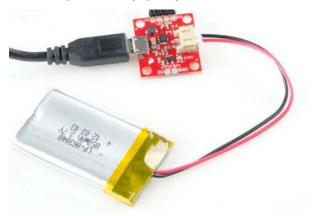
You can also use your own 5V supply and charge over the charge pins labeled '5V' and 'GND.
