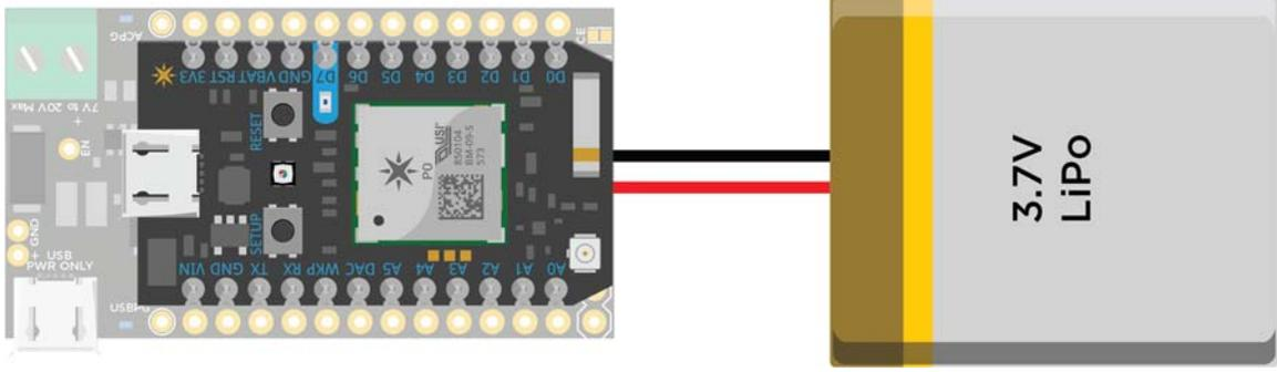
The shield is setup so that when powered from the USB port as well as from a DC supply, it chooses the DC source over USB. The charge current is set to 500mA when charging from USB and set to 1A when charging from a DC source.
