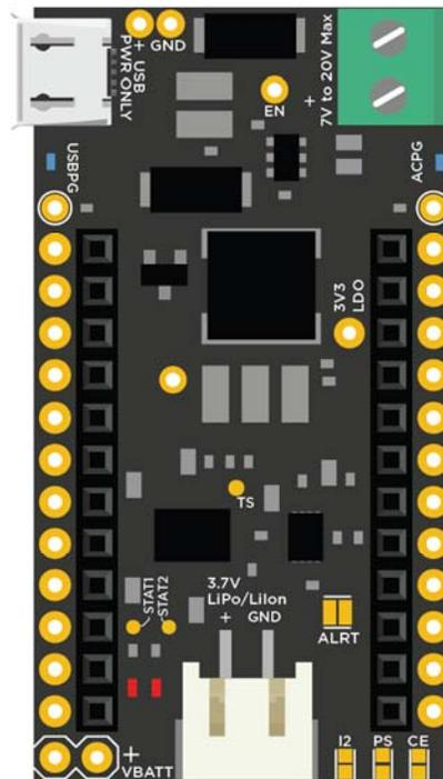
The system switches in between the different power sources automatically, reducing the charge and discharge cycle stress on the battery. The fuel gauge allows you to monitor the battery's state-of-charge (SOC), allowing it to notify the user remotely and take preemptive actions when necessary.
