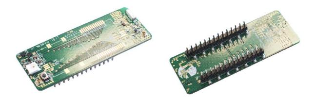
Reference Board used to mount either Pycom OEM modules. Provides the same functionality and pin-out as the developer version of the modules and can be mounted straight-out-of the box.
