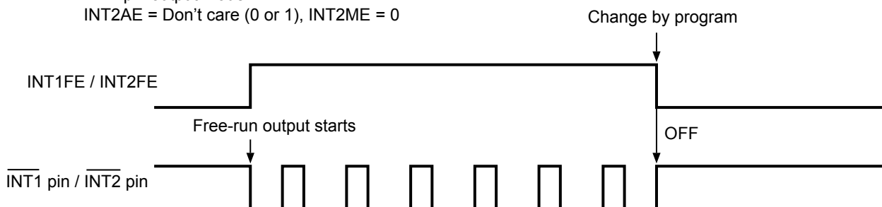
Figure 27 Output Timing of User-set Frequency
