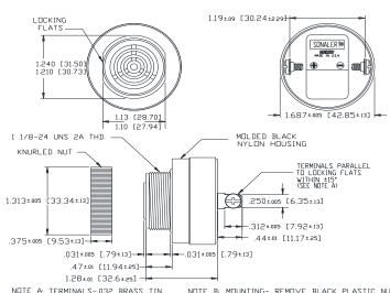
NOTE A: TERMINALS-032 BRASS TIN PLATED, TAPPED FOR #6-32 SCREW. TWO #6-32 NICKEL PLATED BRASS SCREWS INCLUBED. WILL ACCEPT 1/4\* OUICK CONNECT.
