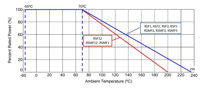
General Purpose Metal Oxide Resistor
